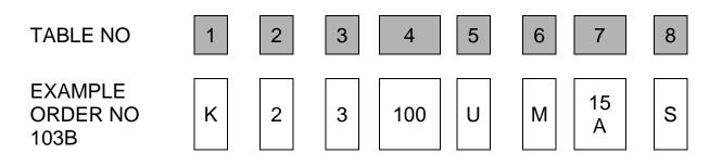
**Example Order No. =** Type 103B T/C-K ; 1/8" sheath diameter ; Inconel 600 sheath material ; 100mm long ; ungrounded measuring junction ; 1/2 N.P.T process connection ; aluminum connection head ; standard calibration.
